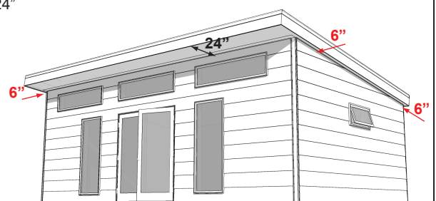
SHORTENED BACK AND SIDE EAVES RECOMMENDED FOR PLACEMENT NEAR REAR & SIDE SET-BACKS
