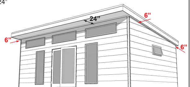
SHORTENED BACK AND SIDE EAVES RECOMMENDED FOR PLACEMENT NEAR REAR & SIDE SET-BACKS
